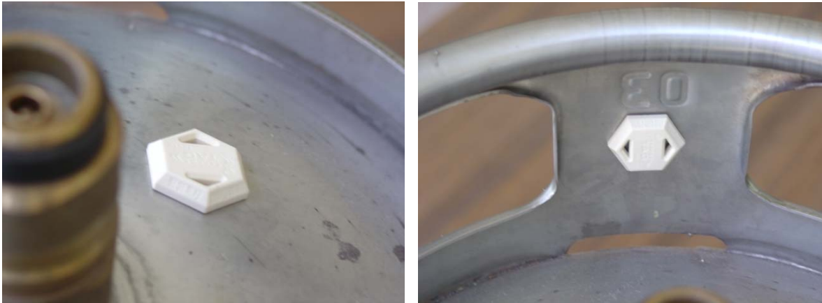
Figure 1. Ferroxtag ATEX certified fixed to metal LPG cylinder through epoxy based adhesive.
